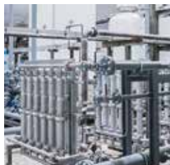
Helium upgrading in Mankota (Canada): The membranes (above) and the plant constructed by Linde.
